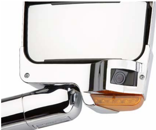
Lower Electronic Module (LEM) with Camera
