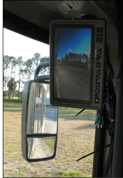
Figure 5-24. Left and right monitor installed next to mirror in portrait orientation
