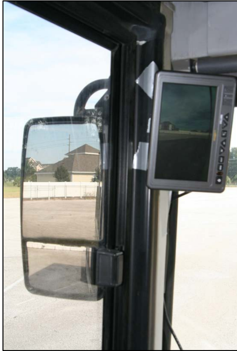
Figure 5-24. Left and right monitor installed next to mirror in portrait orientation
